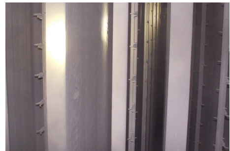
Internal ESP parts
